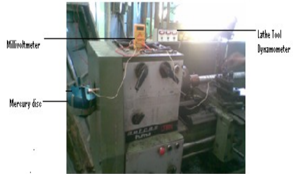
Figure2. Experimental setup for measuring average chip-tool interface Temperature using Tool-work thermo-couple technique [16]
