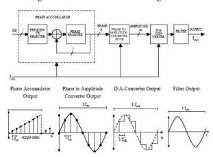
Figure 6. DDS Block Diagram with DAC and Filter
