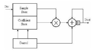
Figure 7. Simplified Block diagram of MAC
