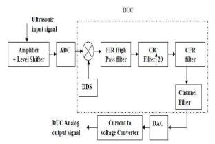
Figure 1. Digital Up Converter Block Diagram
