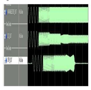
Figure 10. Simulated output of DDS, CIC filter, CFR FIR filter
