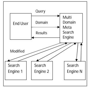
Fig.2. Basic architecture of Proposed MDMSE Model 1
