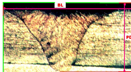
“Fig.1” Schematic of Bead Length and Depth of Penetration
