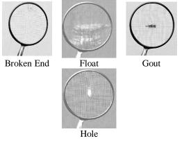
**Figure 2 Weaving defects**
