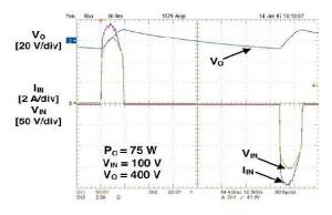
Fig. 12. Measured waveforms of the experimental PFC boost rectifier.  $V_{\rm IN}$  is line voltage,  $I_{\rm IN}$  is line current, and  $V_{\rm O}$  is output voltage.
