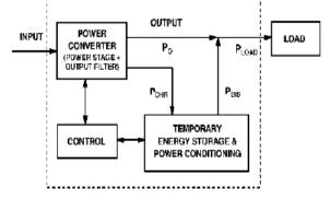
Fig. 2. Conceptual block diagram of the proposed light-load efficiency optimization method.
