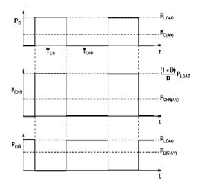
Fig. 3. Timing diagram of output power  $P_{\rm O}$  , charging power  $P_{\rm CHR}$  , and discharging power  $P_{\rm DIS}$  .
