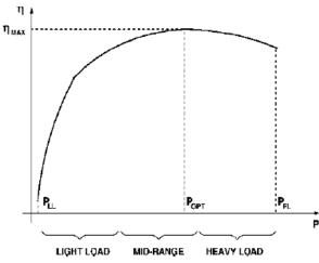
Fig. 1. Typical efficiency profile of a power converter with respect to the power delivered.
