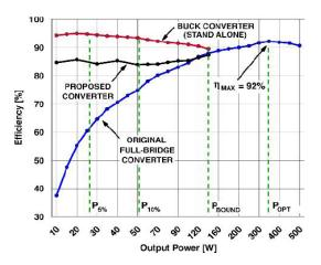
Fig. 10. Measured efficiencies of the original full-bridge converter, the standalone buck converter, and the proposed converter as functions of output power.
