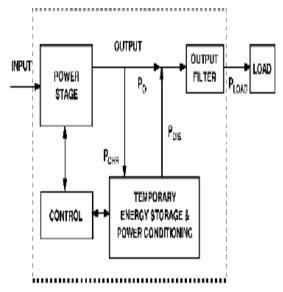
Fig. 5. Conceptual block diagram of another implementation of the proposed light-load efficiency optimization method.
