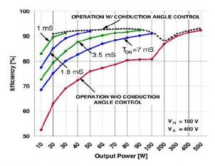
Fig. 13. Measured efficiency of the PFC rectifier as functions of output power for different conduction times  $T_{ON}$ . The dashed line represents efficiency that can be obtained by changing (decreasing)  $T_{ON}$  as output power decreases.
