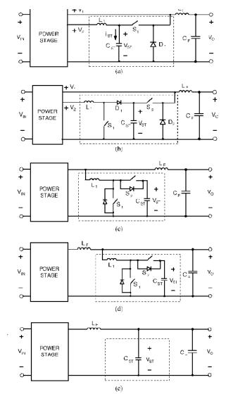
Fig. 6. Examples of circuit implementations of the proposed light-load efficiency optimization method.
