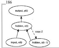
**Figure 1. Architecture of Recurrent Network**
