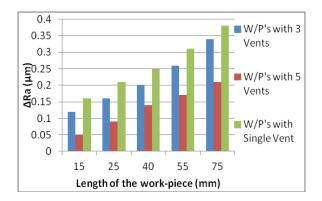
Fig.9.  $\Delta$ Ra in micromachining work-pieces of varying lengths having different vent considerations
