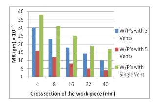
Fig.3. MR in micromachining work-pieces of varying cross sections having different vent considerations
