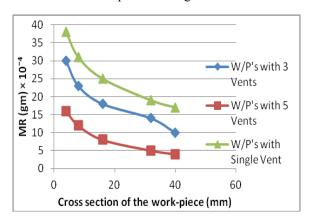
Fig.2. Effect of different vent considerations in work-pieces of varying cross sections on MR
