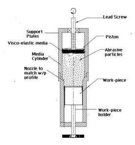
Fig.1 Assembly drawing of the table-top setup for an AFM process
