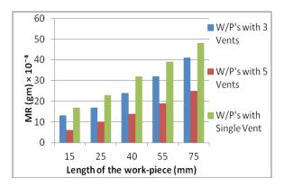
Fig.5. MR in micromachining work-pieces of varying lengths having different vent considerations
