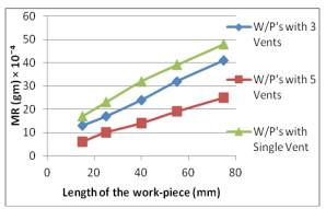
Fig.4. Effect of different vent considerations in work-pieces of varying lengths on MR
