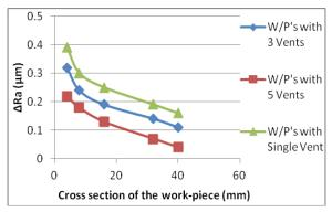
Fig.6. Effect of different vent considerations in work-pieces of varying cross sections on  $\Delta$ Ra
