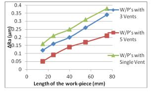
Fig.8. Effect of different vent considerations in work-pieces of varying lengths on  $\Delta Ra$
