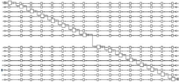
Figure 7. Ripple-carry Incrementer
