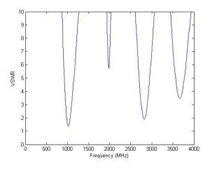
Figure 5 VSWR characteristics of Hybrid Koch fractal antenna
