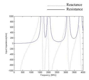
Figure 4 Input impedance characteristics of Hybrid Koch fractal antenna.
