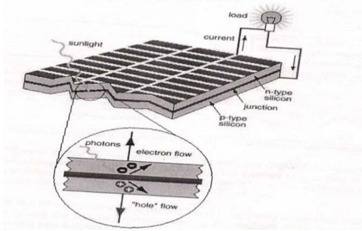
Fig. 1. Electricity generation by solar ( PV) Module
