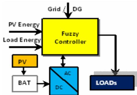
Fig. 3. A control strategy model of an integrated PV-grid/DG integrated power system
