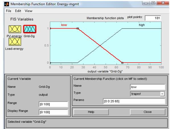
Fig. 8. Membership function for grid/DG time sharing interval i.e. output of the system
