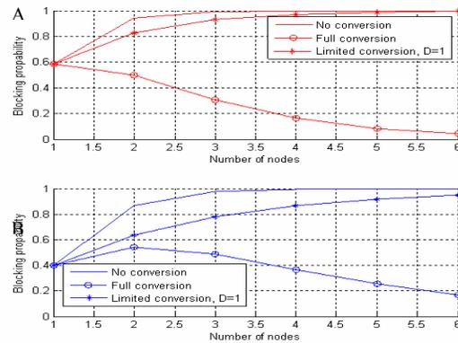
**Figure 11. Blocking Probability Vs No Of Nodes For C=15 Using Heuristic Routing Algorithm A. Long Lightpaths B. Shorter Lightpaths.**
