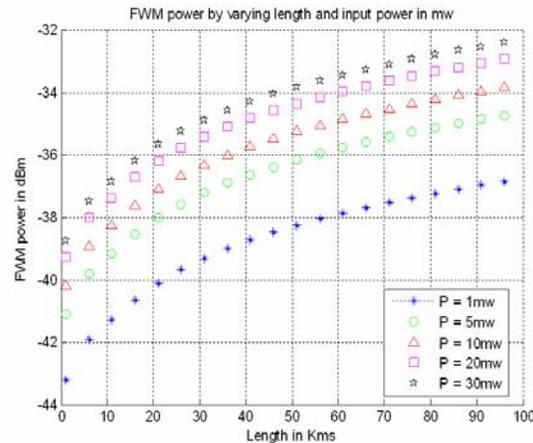
**Figure 3. FWM Noise Power in dBm Vs Length in Kms**
