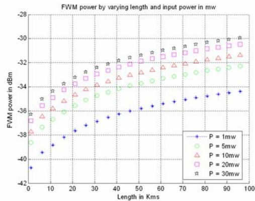
**Figure 6. FWM Noise Power in dBm Vs Length in Kms**
