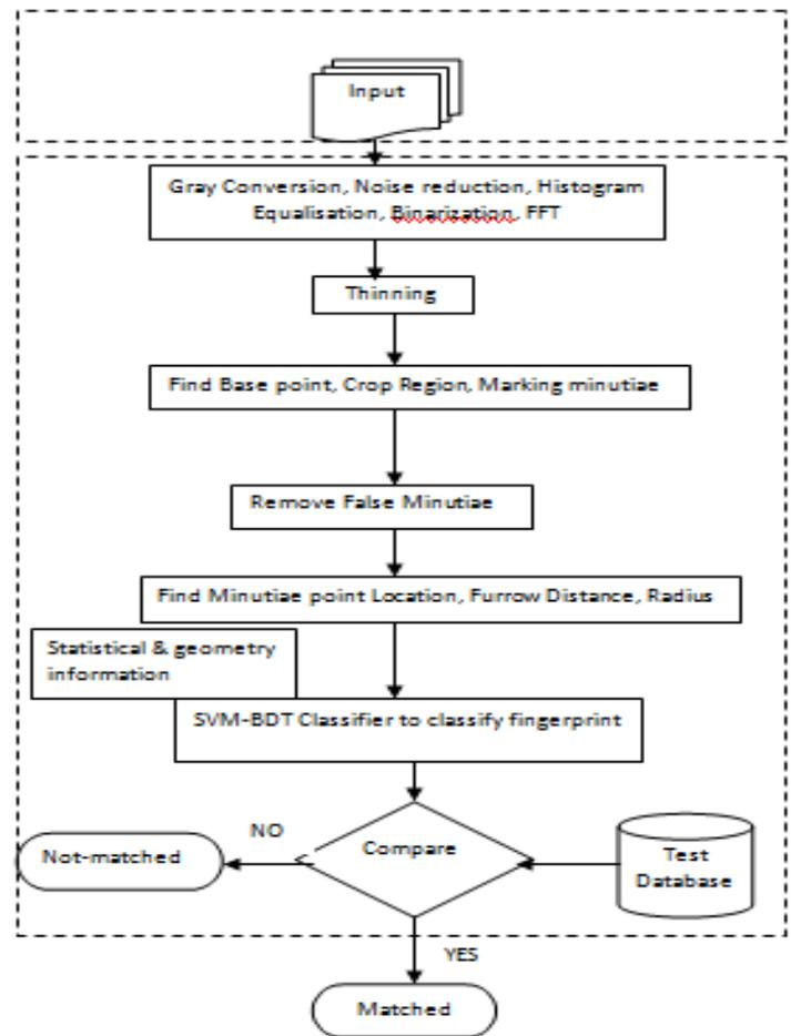
Figure.1 Flow diagram of Proposed IFR system
