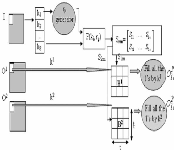
**Figure.4 Hiding Algorithm Flowchart**
