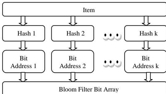
**Figure 1: Inserting an item into a Bloom filter**
