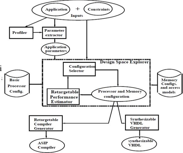
Figure 3: ASSIST (A Scheduler based ASIP Design Methodology)
