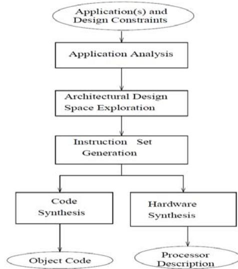
Figure 2: Flow Diagram of ASIP design Methodology
