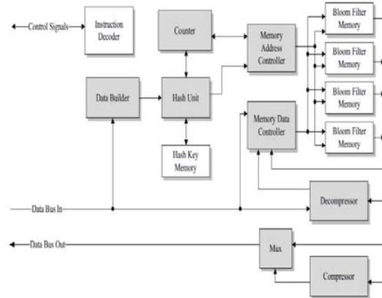
**Figure 7: Bloom filter hardware accelerator hardware flow: arrows indicate the direction of information, shaded blocks indicate modules controlled by the Instruction Decoder.**
