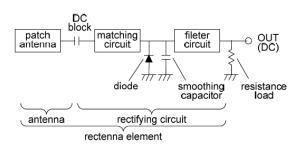
Figure .4. Block diagram of the Rectenna Element
