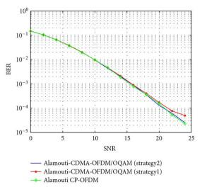
Fig. 9: BER for two complex versions of the Alamouti CDMAOFDM/ OQAM with spreading in time domain, versus Alamouti CP-OFDM for transmission over the 4path frequency selective channel.
