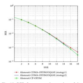
Fig. 10: BER for two complex versions of the Alamouti CDMAOFDM with spreading in time domain, versus Alamouti CP-OFDM for transmission over the 7-path frequency selective channel.
