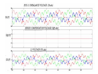
Fig 7: BUS1 voltage, series compensating voltage, and load voltage in Feeder1 under unbalanced source voltage without MC-UPQC.
