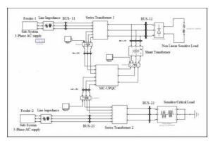
Fig 2: Simulink model of distribution system with MC-UPQC
